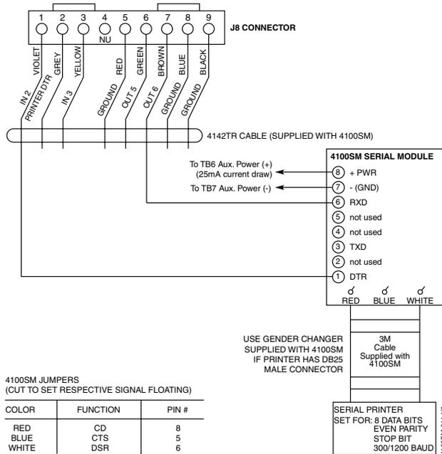
Figure 3-20: 4100SM Using a Serial Printer
