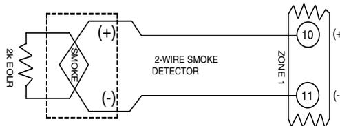
**Figure 3-10: 2-Wire Smoke Detector on Zone 1**
