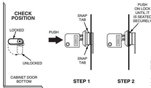
**Figure 3-1: Installing the Lock**
