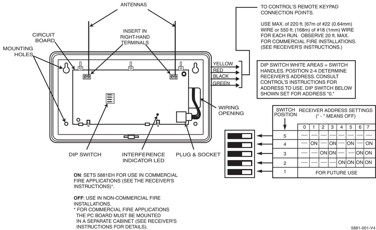
Figure 3-16: RF Receiver (cover removed)
