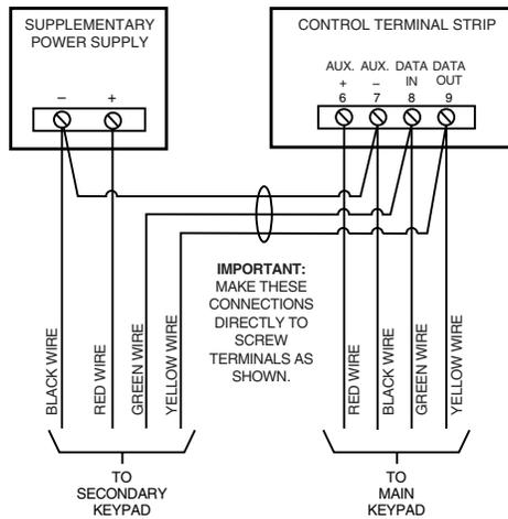
**Figure 3-5: Using a Supplementary Power Supply**
