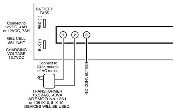
**Figure 3-23: 1361 Transformer and Battery Connections**
