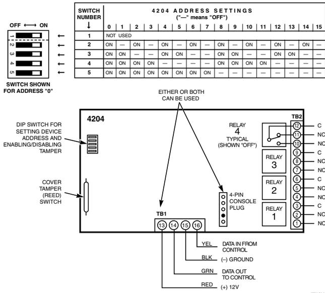
Figure 3-17: 4204 Relay Module
