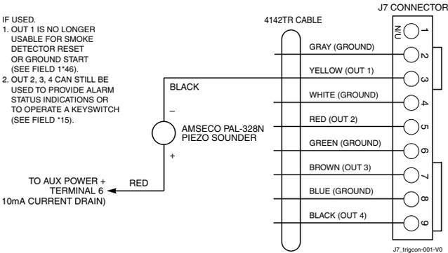
Figure 3-19: Remote Keypad Sounder Wiring
