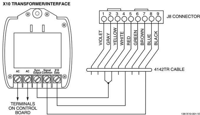
Figure 3-24: 1361X10 Transformer Connections
