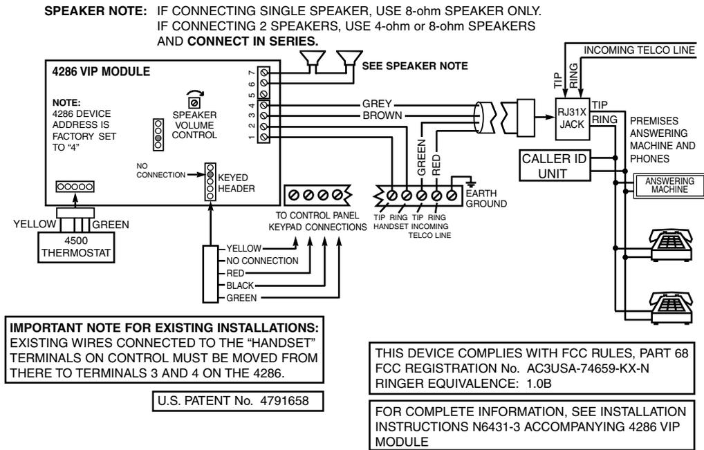
Figure 3-21: VIP Module Connections
