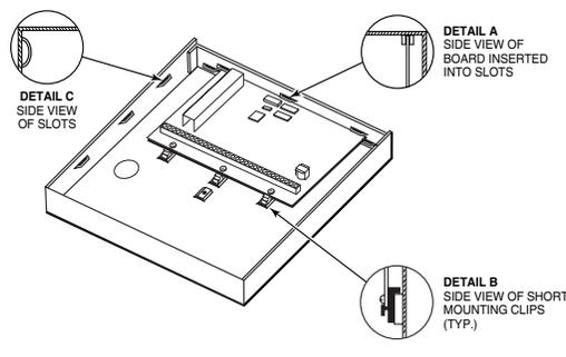
Figure 3-3: Mounting the PC Board
