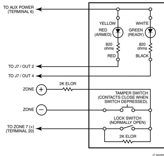
**Figure 3-18: Remote Keyswitch Wiring**
